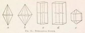
a and b Pyramids, c and d Prisms, owing to the position of the axes a is known as the pyramid of the *first* order and b of the *second* order. Similarly c is the prism of the first order and d of the second order. e is a combination of the forms a, b, c, d, the basal planes being absent.
